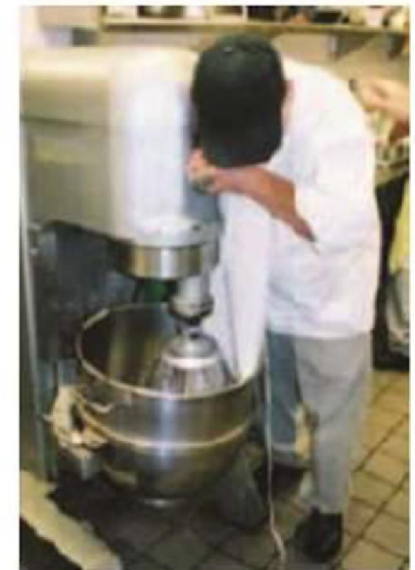
Apron caught in mixer with no guarding
