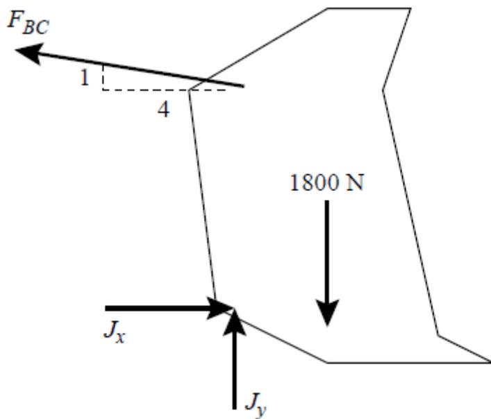
$$\sum M_J : \frac{4}{\sqrt{17}} F_{BC} (0.44 \text{ m}) - \frac{1}{\sqrt{17}} F_{BC} (0.06 \text{ m}) - (1800 \text{ N})(0.2 \text{ m}) = 0$$
