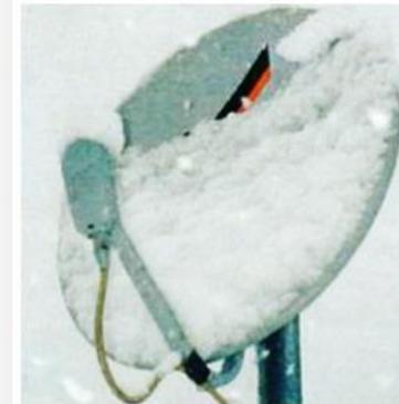
**HIREC® is a super hydrophobic water repellent coating material (similar to paint) developed by NTT to protect its critical telecommunications equipment from snow, ice, and rain interference.**
