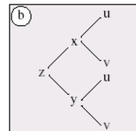
$$\frac{\partial z}{\partial v} = \frac{\partial z}{\partial x} \frac{\partial x}{\partial v} + \frac{\partial z}{\partial y} \frac{\partial y}{\partial v}$$
