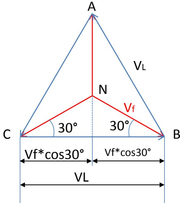
$$V_L = 2 * V_f * \cos 30^\circ = 2 * \frac{\sqrt{3}}{2} V_f \gg V_L = \sqrt{3} V_f$$
