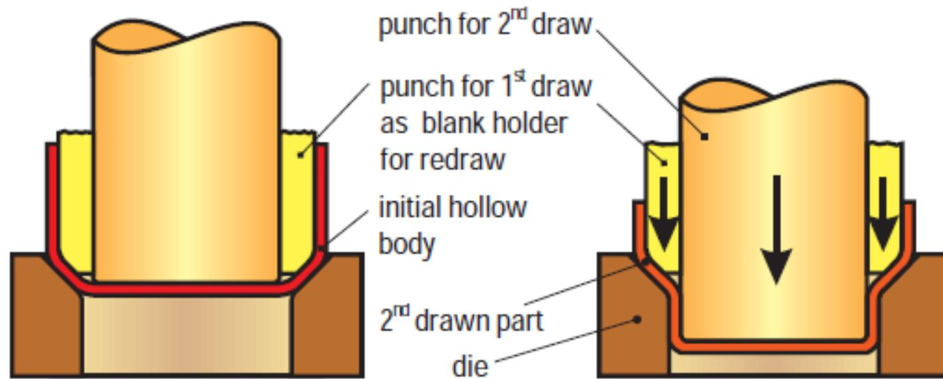
▲ Fig. 2.1.11 Multiple-draw deep drawing with telescopic punch
