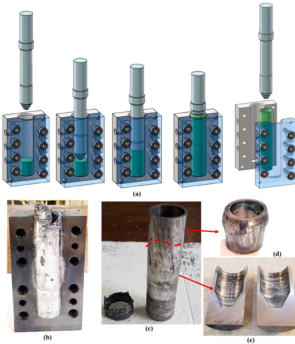
Fig. 1. (a) Schematic presentation of FSE process sequences (b) the fabricated tube inside the mold while the mold half is taken off, (c) the initial section of the pipe is cut as scrap and the rest will be used: (d) the compression test specimen sliced from the tube upside, and (e) the rest of pipe prepared for metallographic investigations.
