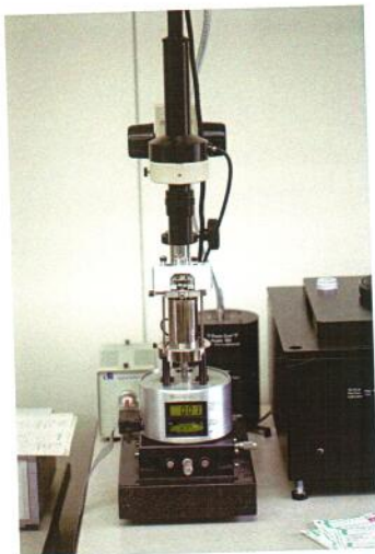
Figure 6.9 An atomic force microscope (AFM) probes the surface of a material to create a three-dimensional image down to the scale of an atom.
