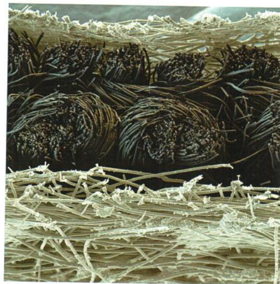
Figure 6.7 A scanning electron microscope (SEM) image of a silver nanoparticle wound dressing made of nylon fabric (white) and an activated charcoal cloth impregnated with silver (black).
